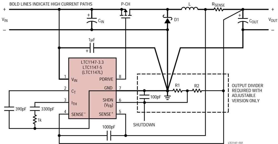
Figure 7. LTC1147 Layout Diagram (See Board Layout Checklist)
