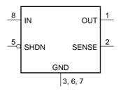
SHDN ; DEVICE INTO SHUTDOWN INPUT
