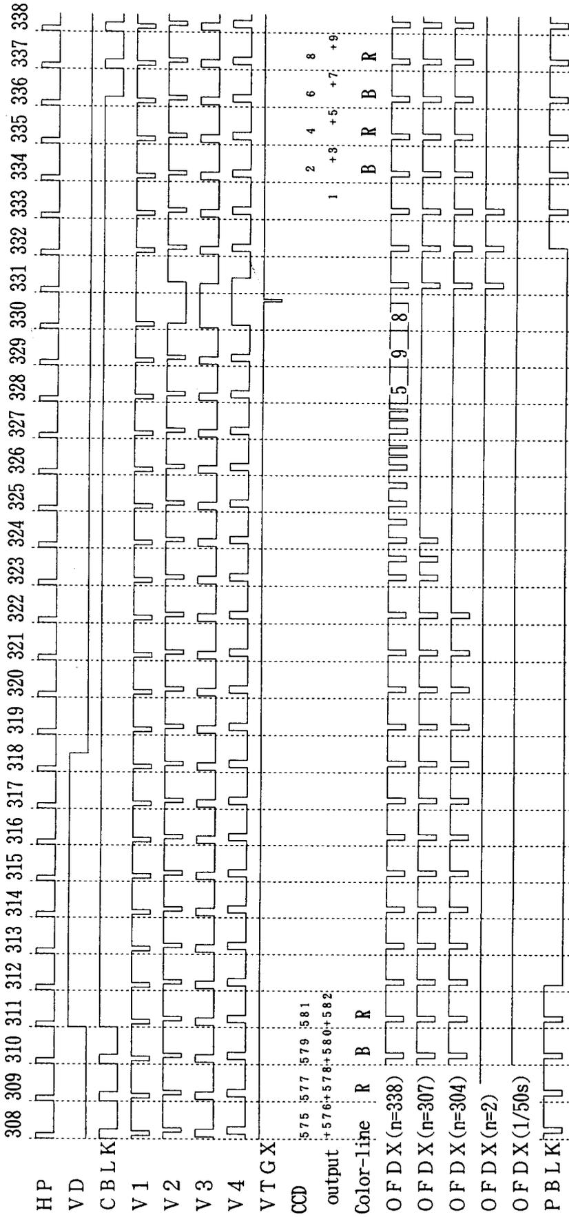
6-2. Horizontal pulse for driving CCD - 1
