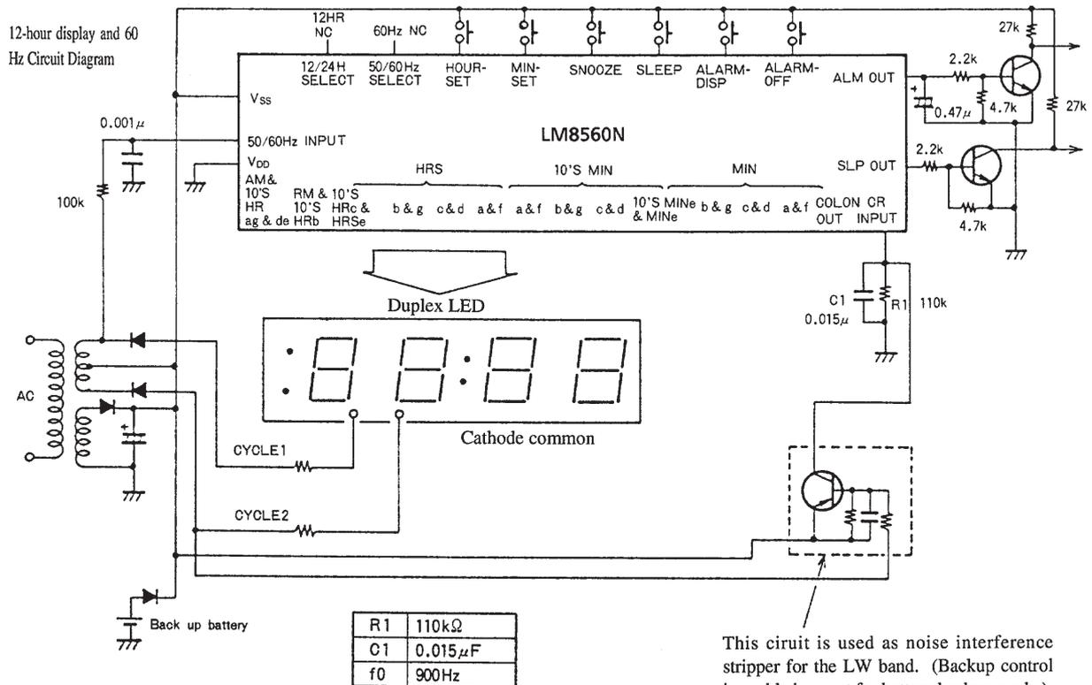
This circuit is used as noise interference stripper for the LW band. (Backup control is enabled except for battery backup mode.)
