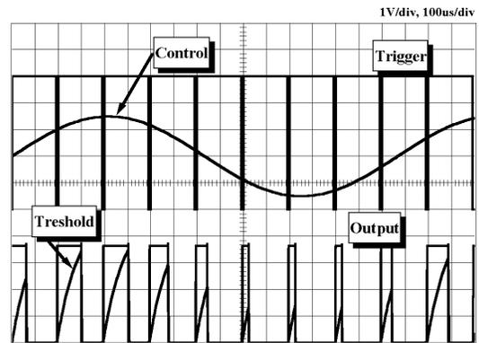
$R_A=9.1k\Omega, R_L=1k\Omega, C1=0.01\mu F, V_{cc}=5V$
