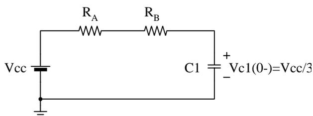
$$C_1 \frac{dv_{c1}}{dt} = \frac{V_{CC} - V(0-)}{R_A + R_B} \quad (1)$$
