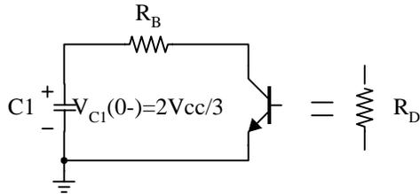
$$C_1 \frac{dv_{C1}}{dt} + \frac{1}{R_A + R_B} V_{C1} = 0 \quad (6)$$
