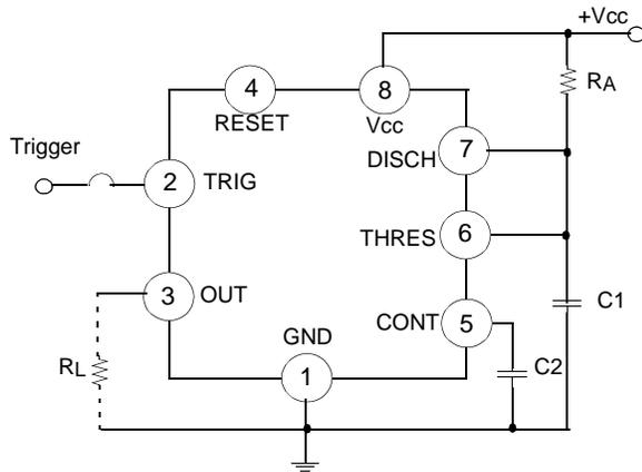
**Figure 1. Monoatable Circuit**
