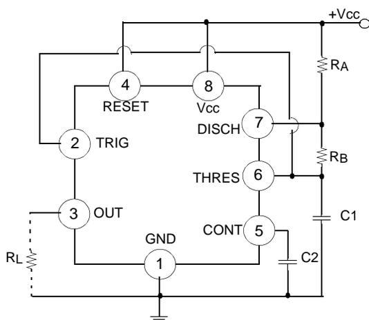
Figure 5. Astable Circuit
