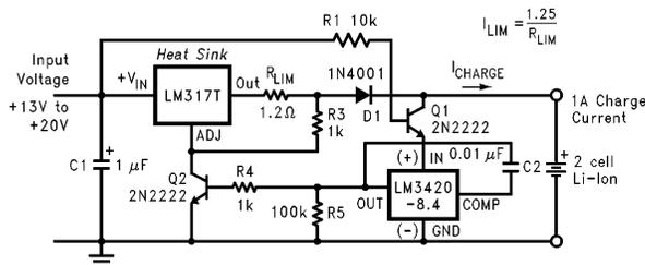
FIGURE 5. Constant Current/Constant Voltage Li-Ion Battery Charger
