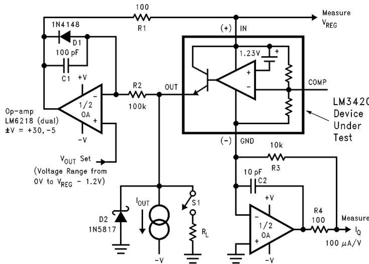
FIGURE 2. LM3420 Test Circuit
