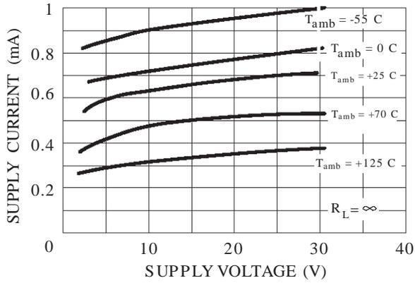
INPUT CURRENT versus SUPPLY VOLTAGE
