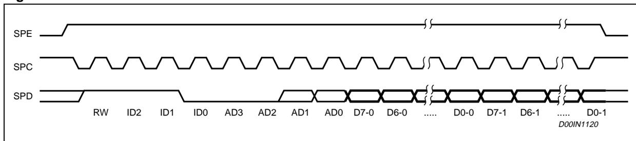
The Read FIFO command consists of 24 clocks or bits.
