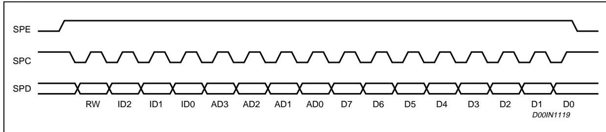
SPE is the Serial Port Enable. It goes high at the start of the transmission and goes back low at the end. SPC is the Serial Port Clock. It is stopped high when SPE is low (no transmission). SPD is the Serial Port Data. It is driven by the falling edge of SPC. It should be captured at the rising edge of SPC.
