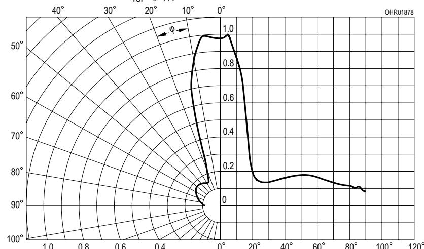
**Radiant intensity**  $\frac{I_e}{I_e 100 \text{ mA}} = f(I_F)$
