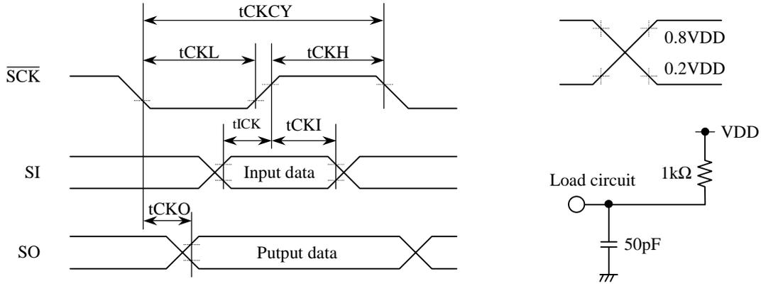
Figure 5 Serial I/O Timing
