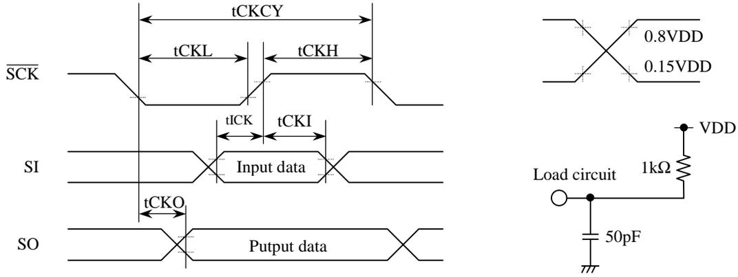
Figure 5 Serial I/O Timing
