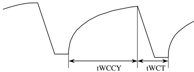
$t_{\text{WCCY}}$  : Charge time due to the external components  $C_w$ ,  $R_w$  and  $R_l$ .
