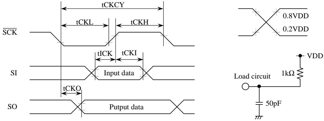
Figure 5 Serial I/O Timing
