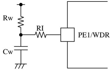
tWCCY : Charge time due to the external components Cw, Rw and R1.
