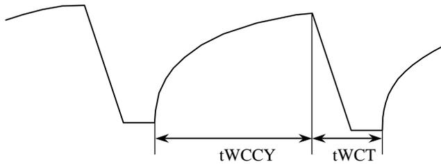
TWCCY : Charge time due to the external components Cw, Rw and Rl.
