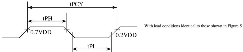
Figure 6 Port PE0 Pulse Output Timing
