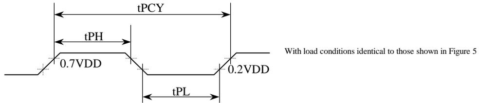
Figure 6 Port PE0 Pulse Output Timing
