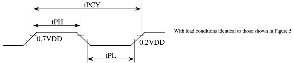
Figure 6 Port PE0 Pulse Output Timing
