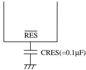
Figure 4 Reset Circuit
