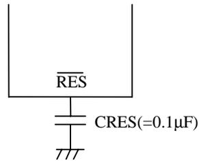
Figure 4 Reset Circuit
