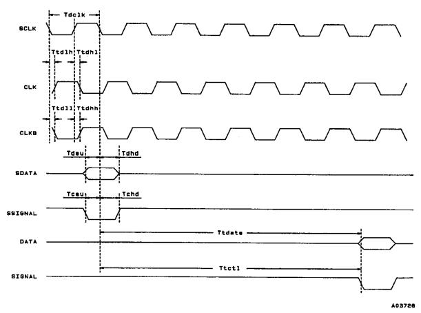
SSIGNAL refers to the SHDEN, SCTL, BYPASS and PWRSV signals. SIGNAL refers to the HDEN and CTL signals.
