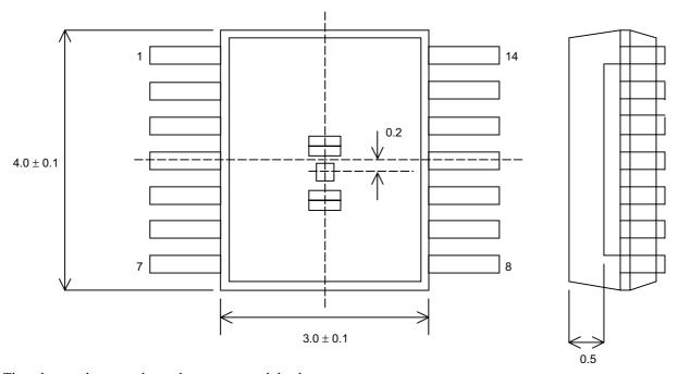
The tolerance between the package center and the detector pattern center :
