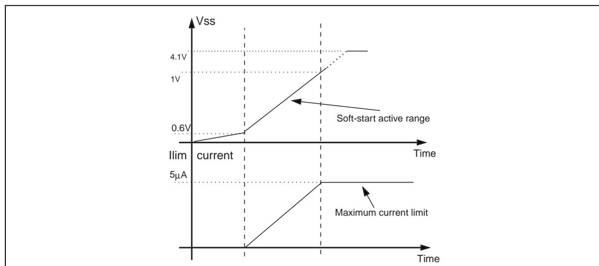
Because the system implements the soft start controlling the inductor current, the soft start capacitor selection is function of the output capacitance, the current limit and the soft start active range ( $\Delta V_{SS}$ ).
