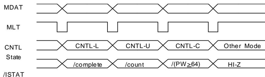
Fig.3. /ISTAT output signal according to CNTL Register
