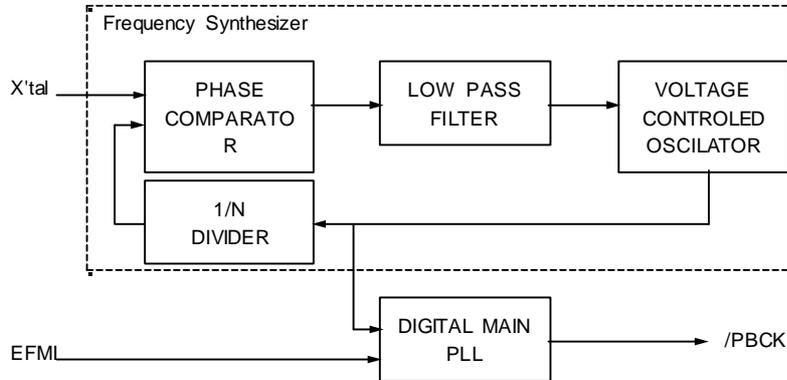
Fig.17. Digital PLL circuit diagram
