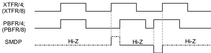
Fig.14. Timing chart of SMDP output
