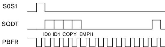
Fig.12. Timing chart of channel status data output
