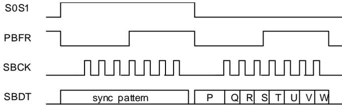
Fig.11. Timing chart of digital audio output
