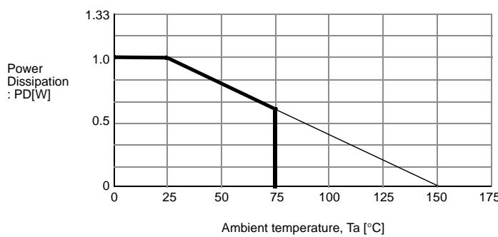
Power dissipation decreases at the rate of 13.6mV / °C when mounted on 30mm × 30mm × 1.5mm PCB (Phenolic resin material) and used above Ta=25°C.
