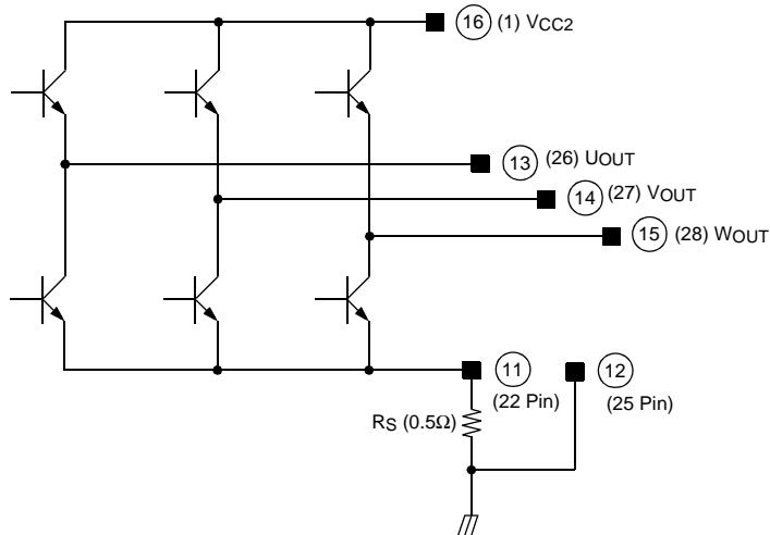
The RS (Output current sensing resistor) is connected to GOUT and Approx. 0.5Ω. It converts motor current to a voltage which is feedback amplifier.
