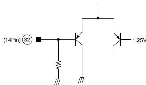
Forward mode:  $V_{FRCTL} \geq 1.8V$
