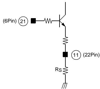
The input voltage range is 2V ≤ V<sub>REF</sub> ≤ (V<sub>CC1</sub> - 2V).
