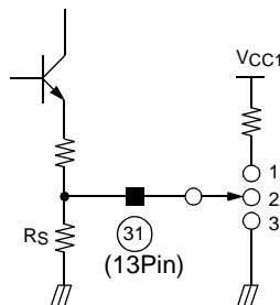
The motor torque ripple is controlled by the TRCTL (Torque ripple control) voltage as follows.
