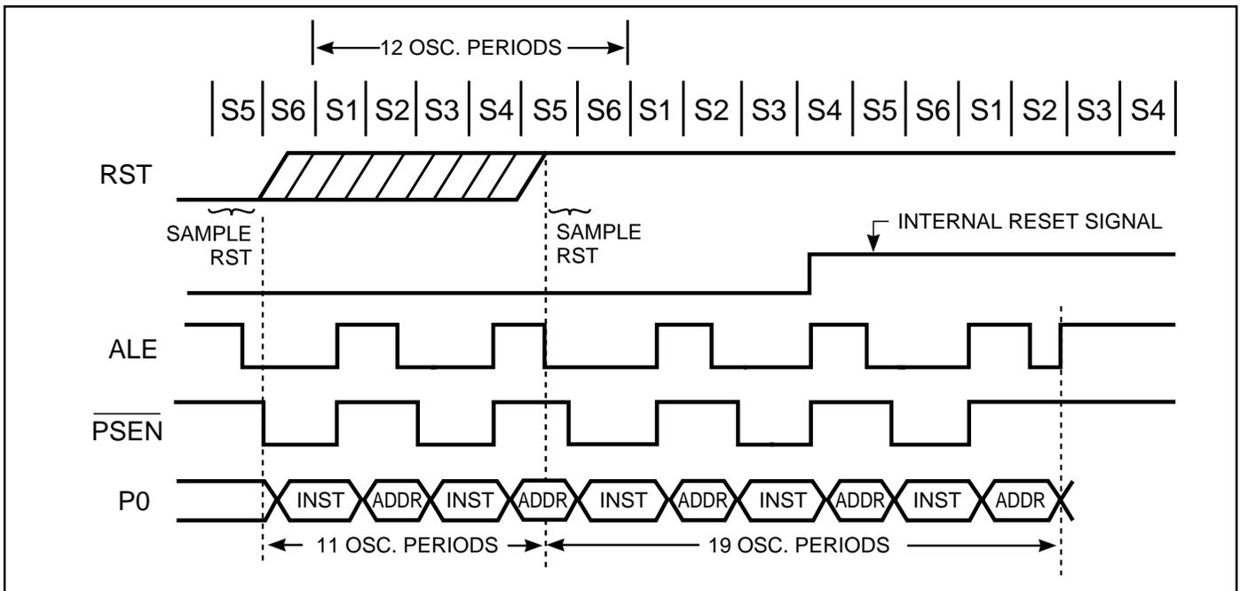
**Figure 21. Reset Timing**
