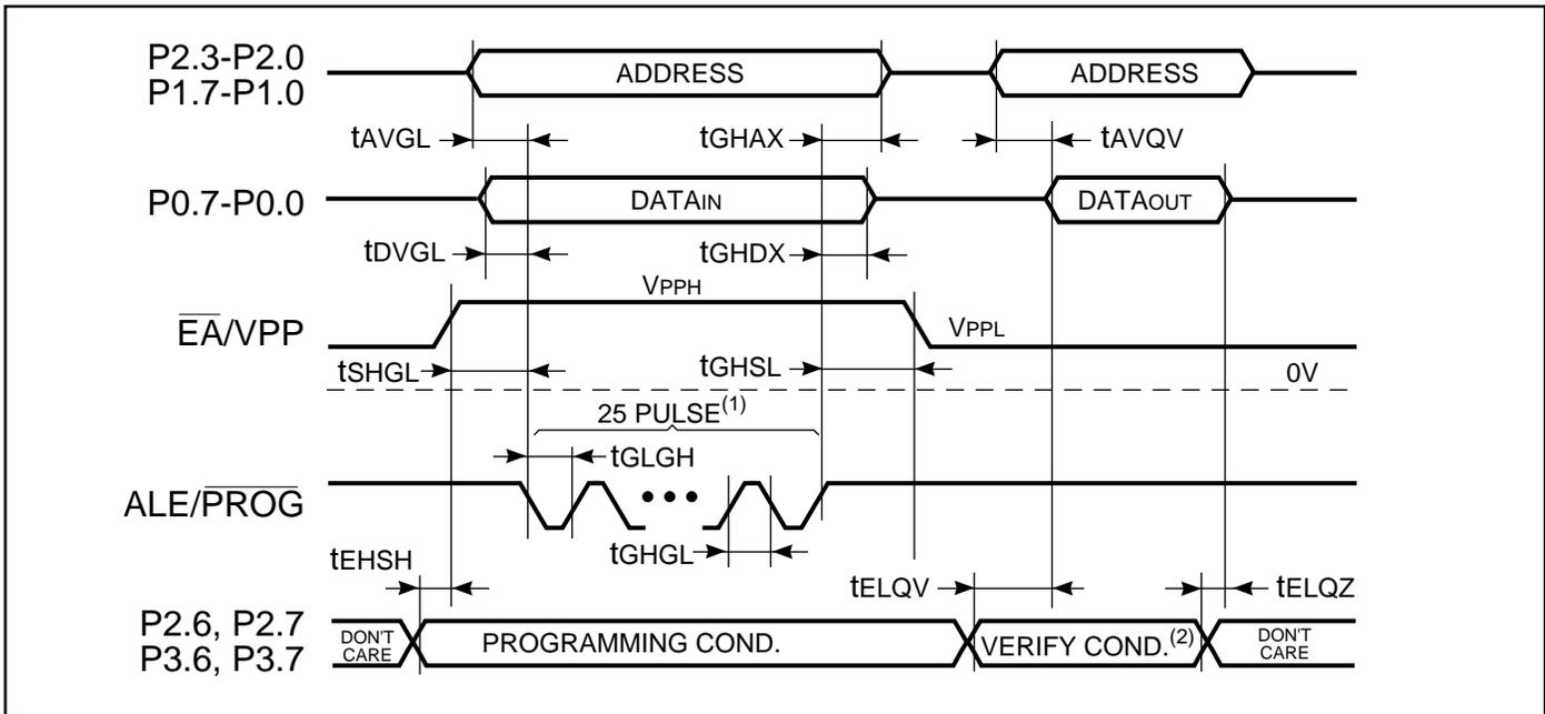
Figure 29. Flash Memory Programming and Verification Timing Waveform
