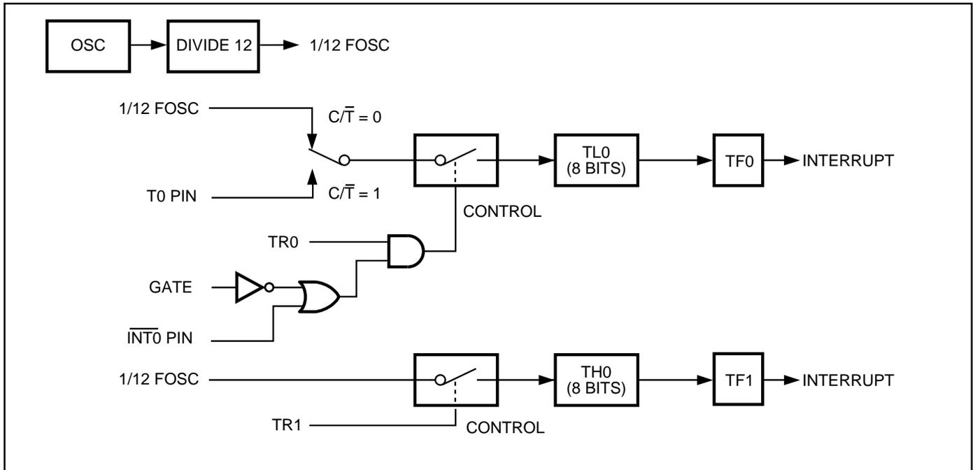
Figure 11. Timer/Counter 0 Mode 3: Two 8-Bit Counters
