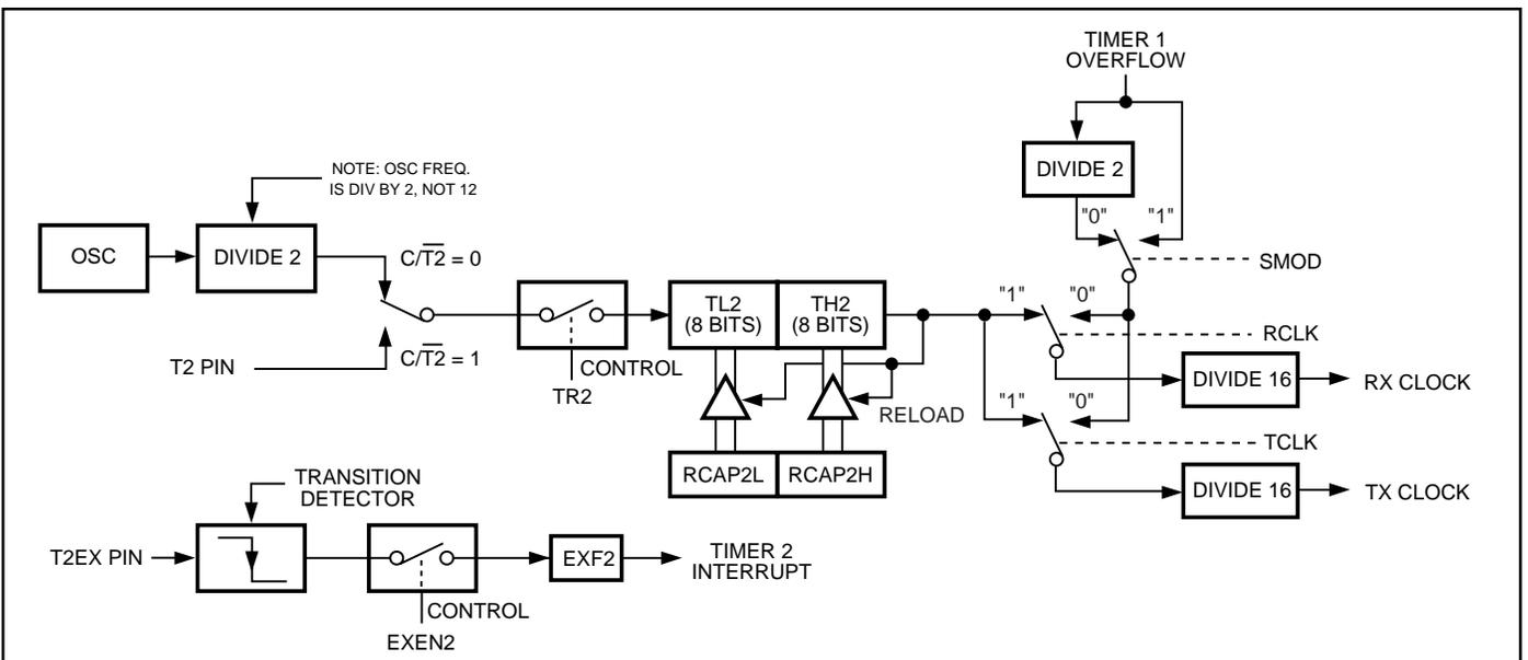
Figure 14. Timer 2 in Baud Rate Generator Mode
