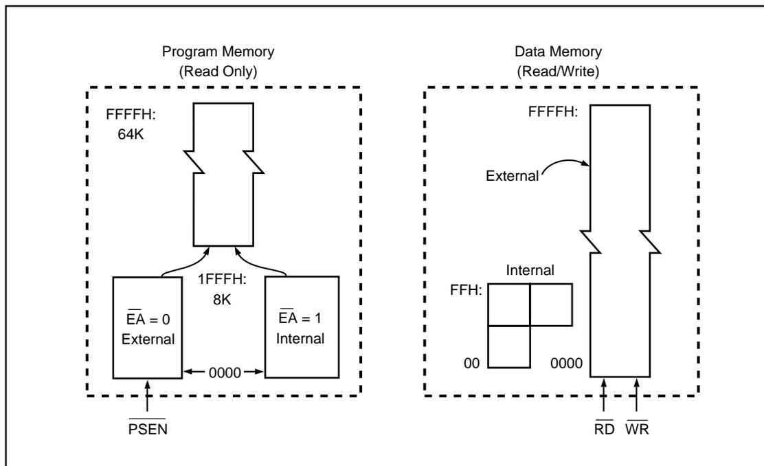
Figure 5. IS89C52 Program and Data Memory Structure
