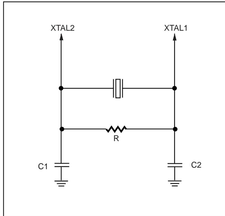
Figure 26. Oscillator Connections for High Speed (> 24 MHz)
