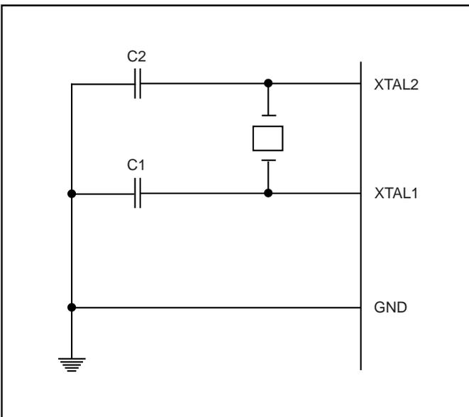
Figure 21. Oscillator Connections
