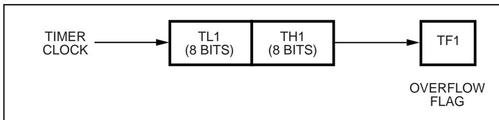
Figure 9. Timer/Counter 1 Mode 1: 16-Bit Counter
