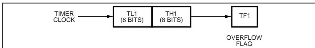
**Figure 9. Timer/Counter 1 Mode 1: 16-Bit Counter**
