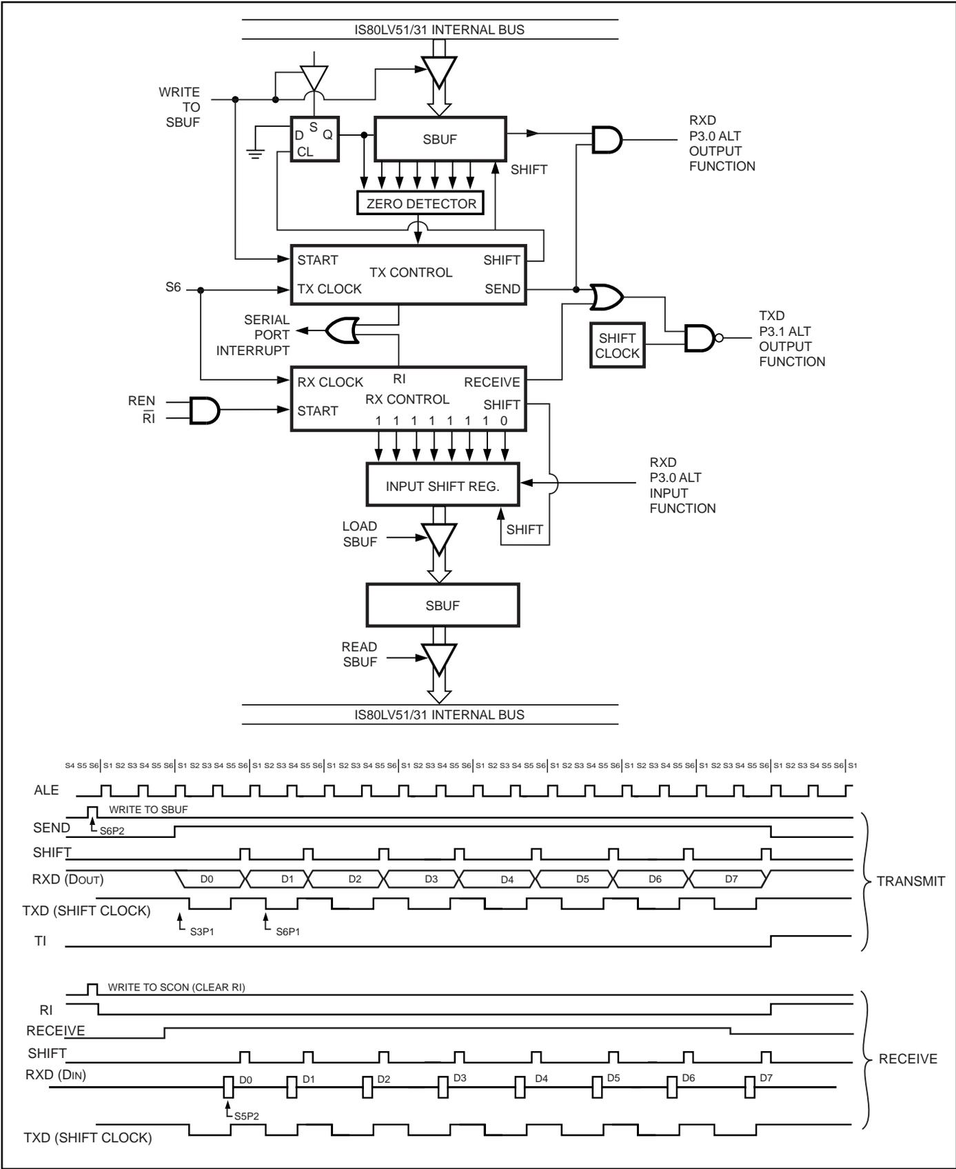
Figure 12. Serial Port Mode 0
