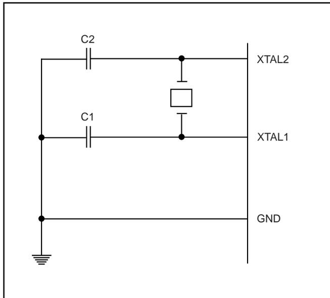
Figure 21. Oscillator Connections
