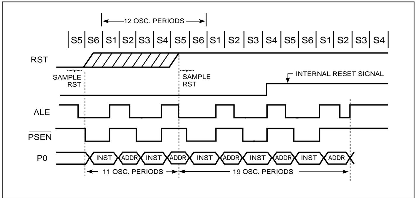
**Figure 19. Reset Timing**
