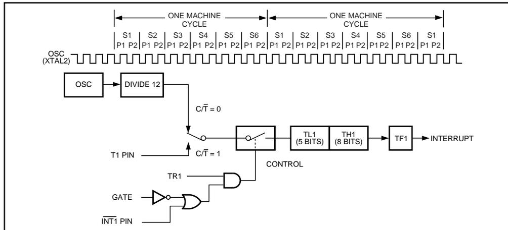
**Figure 8. Timer/Counter 1 Mode 0: 13-Bit Counter**
