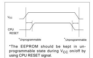
In addition, when V<sub>CC</sub> is turned on or off, the input level of control pins must be held as shown in the table below.
