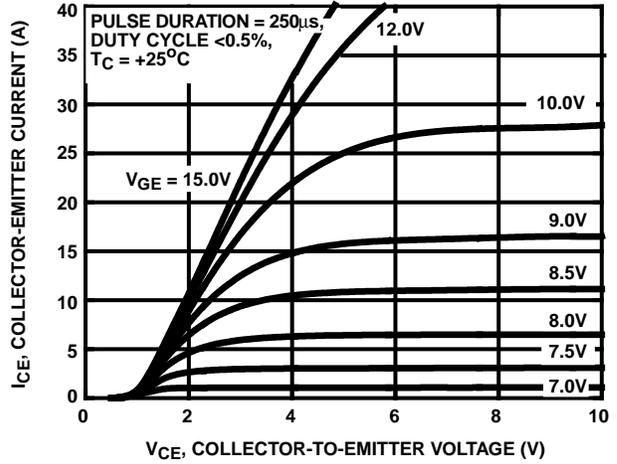
FIGURE 2. SATURATION CHARACTERISTICS
