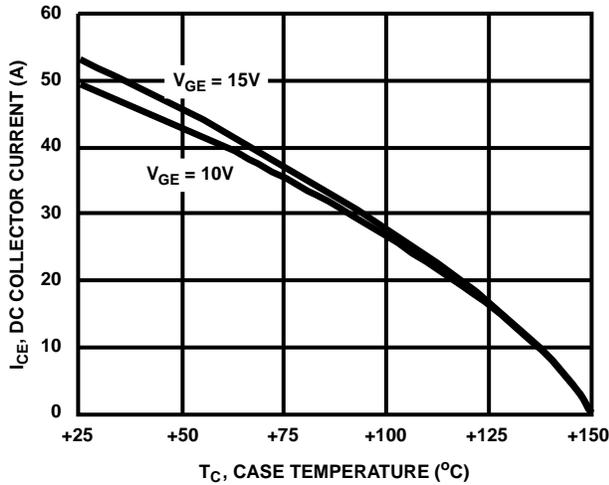
FIGURE 3. MAXIMUM DC COLLECTOR CURRENT vs CASE TEMPERATURE
