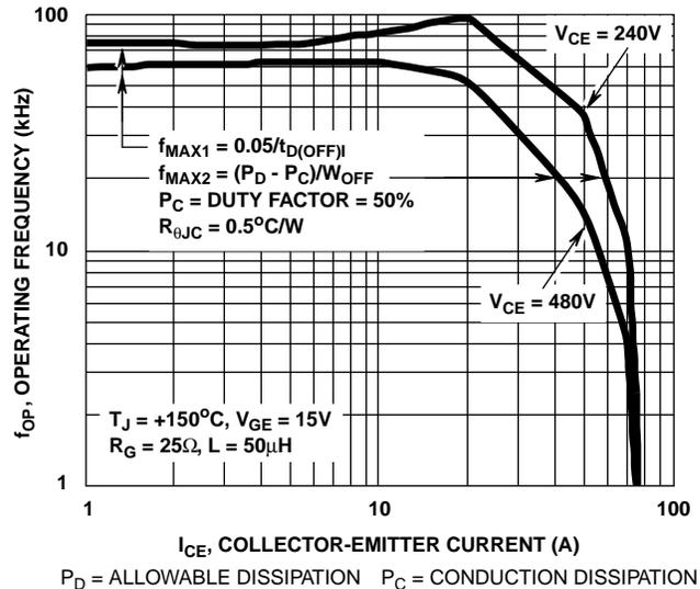
FIGURE 10. OPERATING FREQUENCY vs COLLECTOR-EMITTER CURRENT AND VOLTAGE
