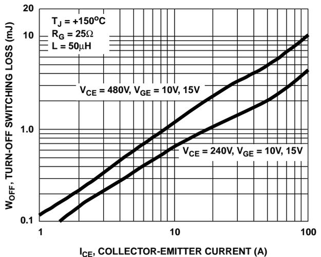
FIGURE 8. TURN-OFF SWITCHING LOSS vs COLLECTOR-EMITTER CURRENT
