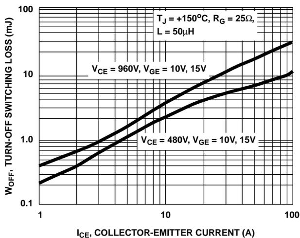
FIGURE 8. TURN-OFF SWITCHING LOSS vs COLLECTOR-EMITTER CURRENT
