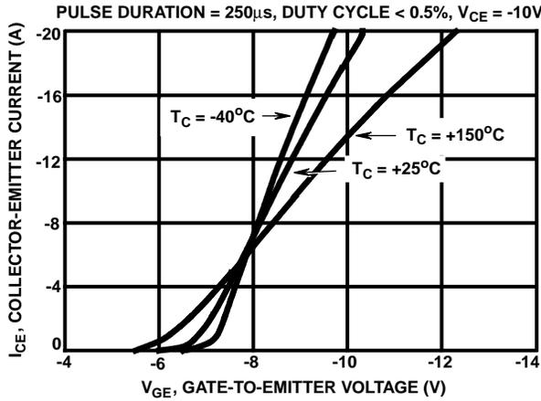
FIGURE 1. TRANSFER CHARACTERISTICS
