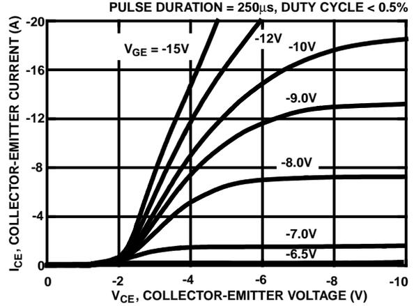
FIGURE 2. SATURATION CHARACTERISTICS
