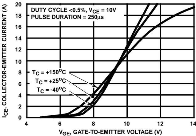
FIGURE 1. TRANSFER CHARACTERISTICS
