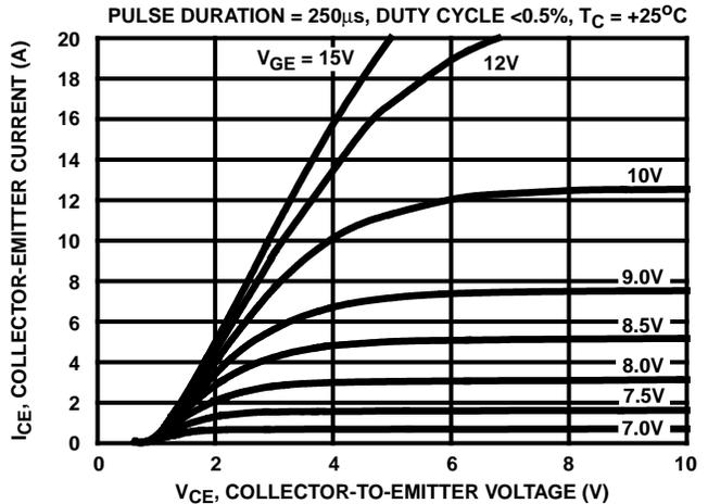
FIGURE 2. SATURATION CHARACTERISTICS
