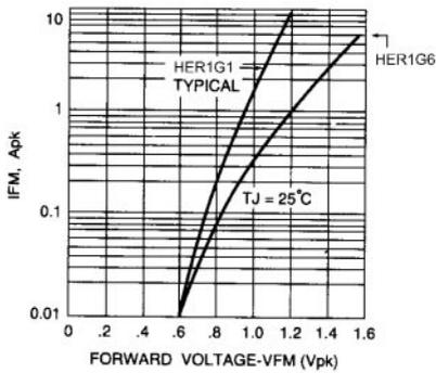
Fig. 2 - FORWARD CHARACTERISTICS
