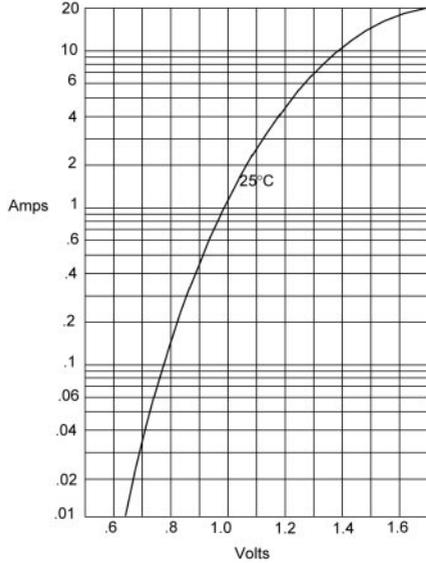
Instantaneous Forward Current - Amperes *versus*
