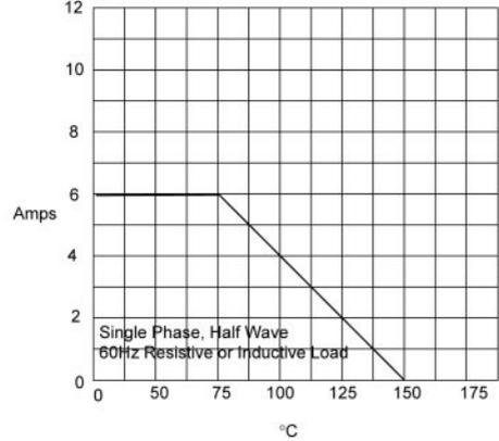
Average Forward Rectified Current - Amperes *versus*
