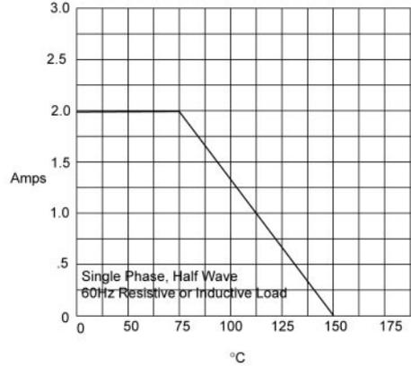
Average Forward Rectified Current - Amperes *versus*
