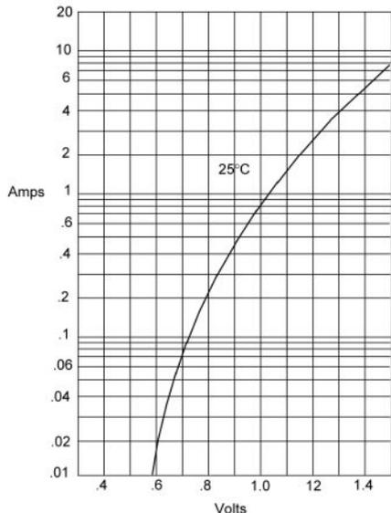
Instantaneous Forward Current - Amperes *versus*
