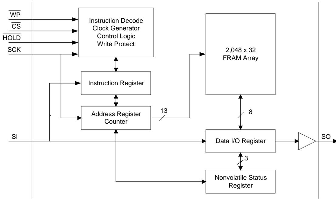
Figure 1. Block Diagram
