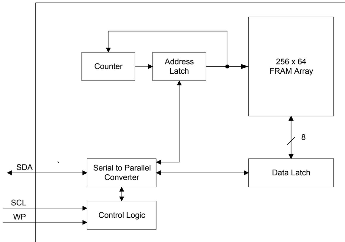
Figure 1. Block Diagram
