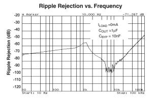
**Ripple Rejection vs. Frequency**
