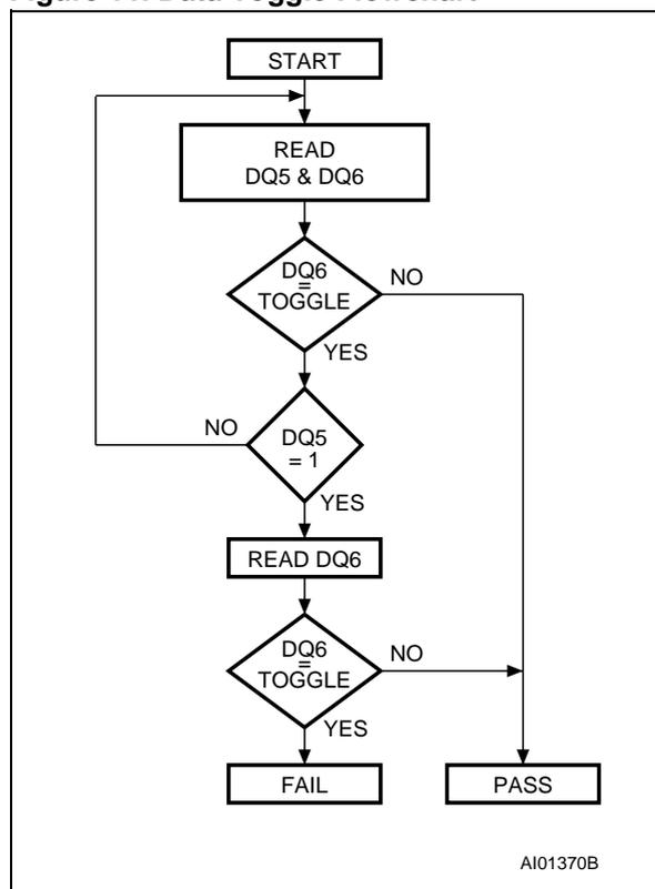
The Error Flag (DQ5) bit is set if either an internal time-out occurred while the embedded algorithm attempted to program the byte, or if the DSP attempted to program a 1 to a bit that was not erased (not erased is logic 0).
