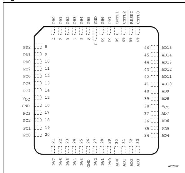
Figure 4. PQFP Connections
