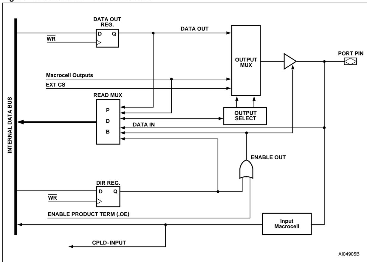
As shown in Figure 19, the ports contain an output multiplexer whose select signals are driven by the configuration bits determined by PSDsoft Express. Inputs to the multiplexer include the following:
