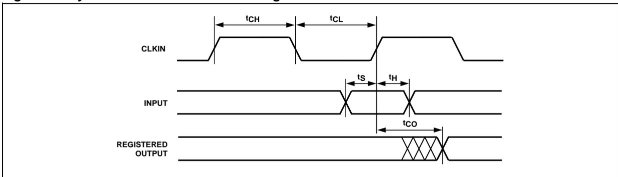
Figure 32. Asynchronous Clock Mode Timing (product term clock)
