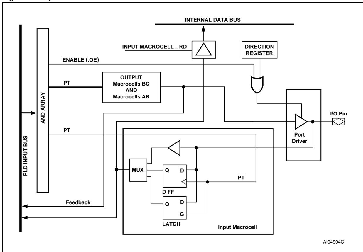
**Input Macrocells (IMC).** The CPLD has 16 Input Macrocells (IMC), one for each pin on Ports B and C. The architecture of the IMCs is shown in Figure 18. The IMCs are individually configurable, and can be used as a latch, a register, or to pass incoming Port signals prior to driving them onto the PLD input bus. This is useful for sampling and debouncing inputs to the AND array (keypad inputs, etc.). Additionally, the outputs of the IMCs can be read by the DSP asynchronously at any time
