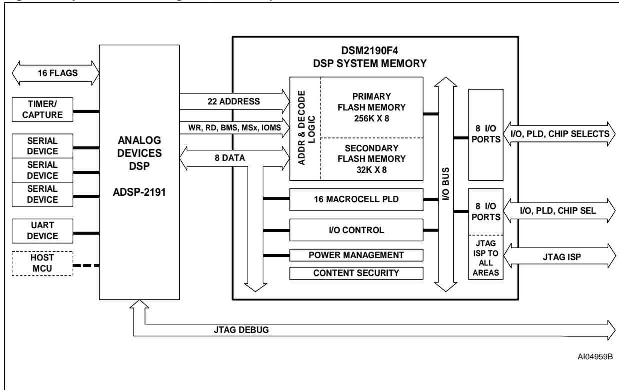
The two-chip combination of a DSP and a DSM device is ideal for systems which have limitations on size, EMI levels, and power consumption. DSM memory and logic are “zero-power”, meaning they automatically go to standby between memory accesses or logic input changes, producing low active and standby current consumption, which is ideal for battery powered products.
