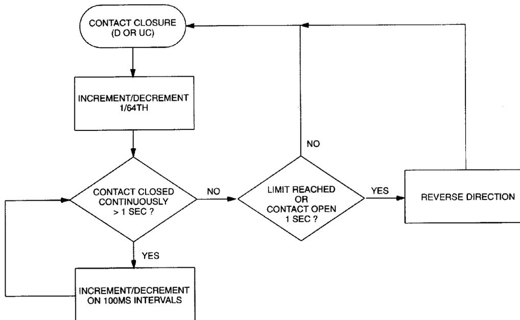
CONTACT OPEN AND CONTACT CLOSURE TIMING IS  $1s \pm 15\%$ .
