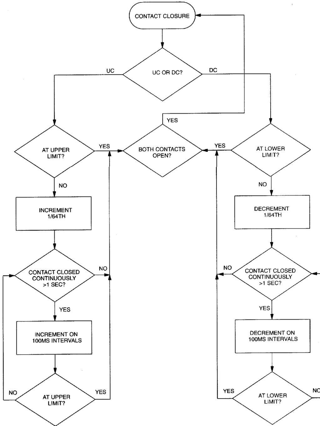
CONTACT OPEN AND CONTACT CLOSURE TIMING IS 1sec. ± 15%.
