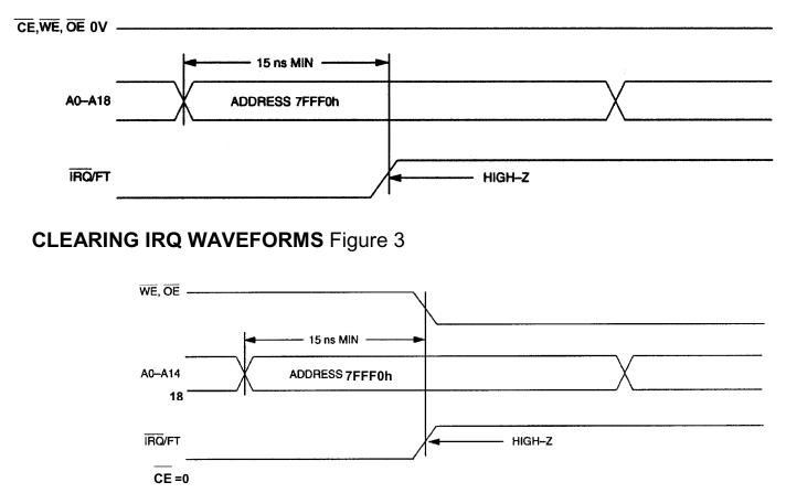
The  $\overline{IRQ}/FT$  pin can also be activated in the battery backed mode. The  $\overline{IRQ}/FT$  will go low if an alarm occurs and both ABE and AE are set. The ABE and AE bits are cleared during the power-up transition, however an alarm generated during power-up will set AF. Therefore the AF bit can be read after system power-up to determine if an alarm was generated during the power-up sequence. Figure 4 illustrates alarm timing during the battery back-up mode and power-up states.
