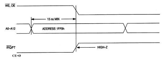
The IRQ/FT pin can also be activated in the battery backed mode. The IRQ/FT will go low if an alarm occurs and both ABE and AE are set. The ABE and AE bits are cleared during the power-up transition, however an alarm generated during power-up will set AF. Therefore the AF bit can be read after system power-up to determine if an alarm was generated during the power-up sequence. Figure 4 illustrates alarm timing during the battery back-up mode and power-up states.
