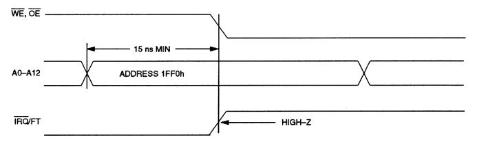
The IRQ/FT pin can also be activated in the battery-backed mode. The IRQ/FT will go low if an alarm occurs and both ABE and AE are set. The ABE and AE bits are cleared during the power-up transition, however an alarm generated during power-up will set AF. Therefore the AF bit can be read after system power-up to determine if an alarm was generated during the power-up sequence. Figure 4 illustrates alarm timing during the battery backup mode and power-up states.
