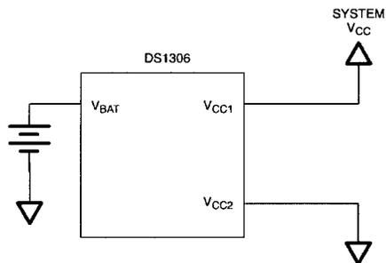
Note: Device is write protected if  $V_{CC} < V_{CCTP}$
