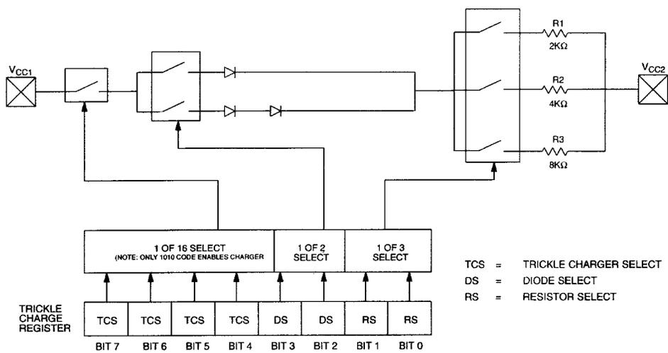
**TRICKLE CHARGER RESISTOR & DIODE SELECT Table 2**
