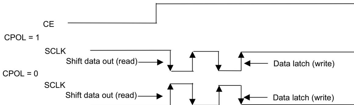
CPHA bit polarity in the processor (if applicable) may need to be set accordingly.
