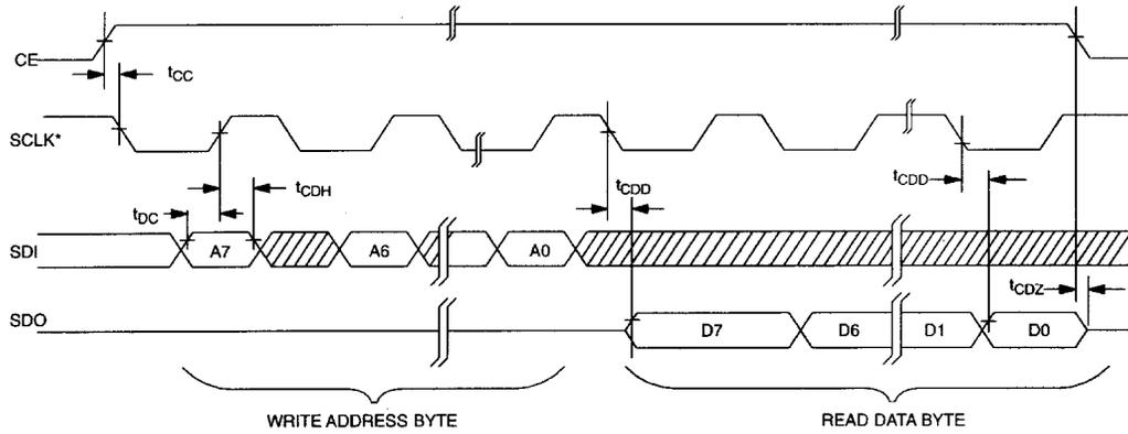
**TIMING DIAGRAM: SPI WRITE DATA TRANSFER Figure 13**
