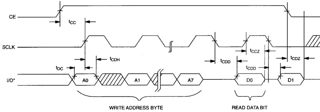
**TIMING DIAGRAM: 3-WIRE WRITE DATA TRANSFER** Figure 11
