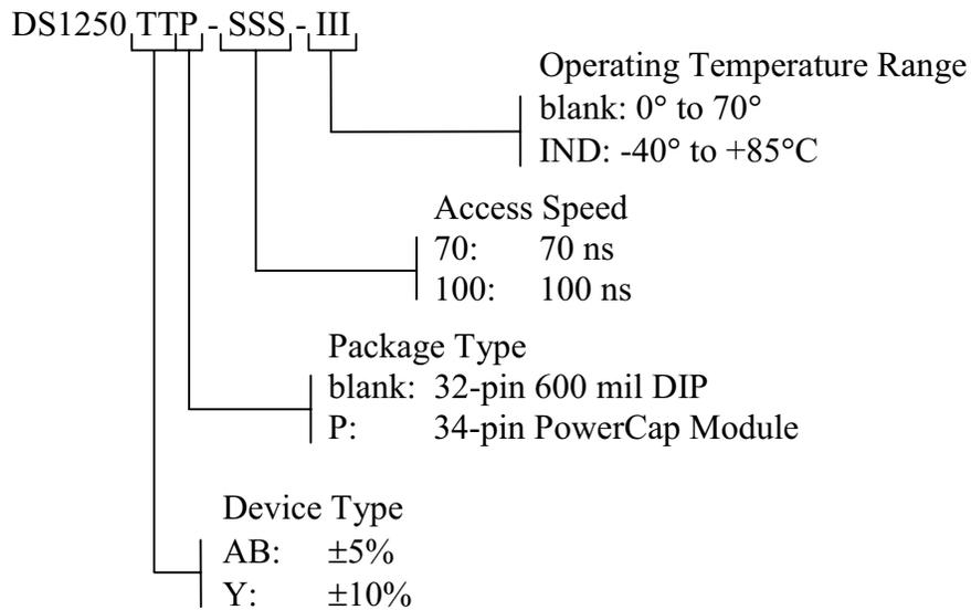
**DS1250Y/AB NONVOLATILE SRAM, 32-PIN, 740 MIL-EXTENDED DIP MODULE**
