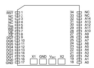
34-Pin PowerCap Module Board (Uses DS9034PCX PowerCap)
