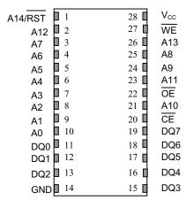
28-Pin Encapsulated Package 740mil Extended
