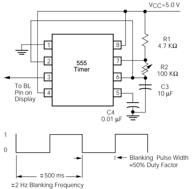
**Figure 4. DLX2416 Dimming circuit using a 556 and Dimming (Blanking) timing**
