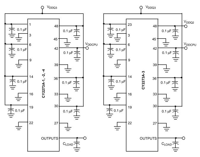
Note: All Capacitors must be placed as close to the pins as is possible
