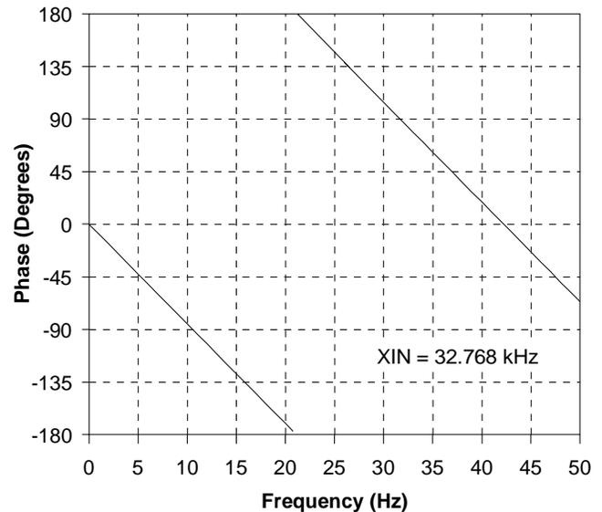
Figure 7. Filter Phase Plot to 50 Hz
