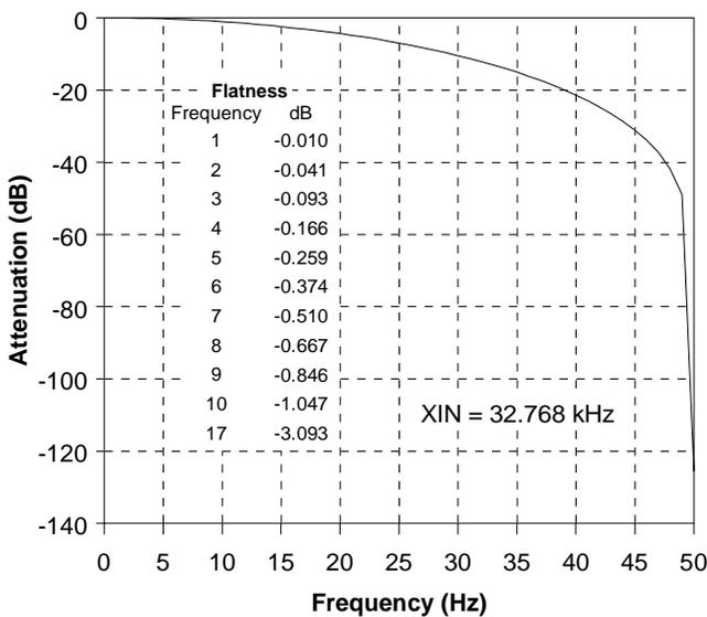
Figure 6. Filter Magnitude Plot to 50 Hz
