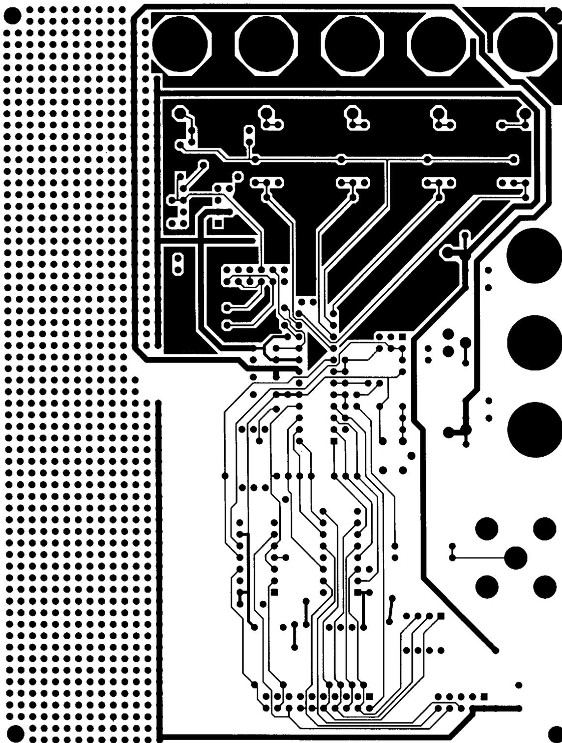
Figure 5. Bottom Trace Layer (NOT TO SCALE)
