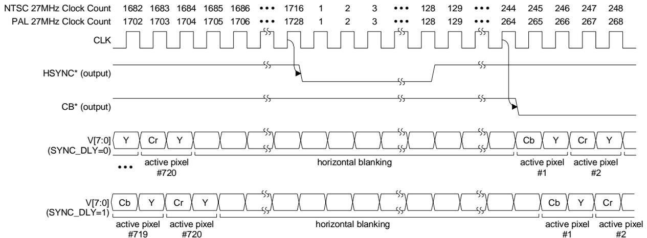
**Figure 7. CCIR601 Input Master Mode Horizontal Timing**
