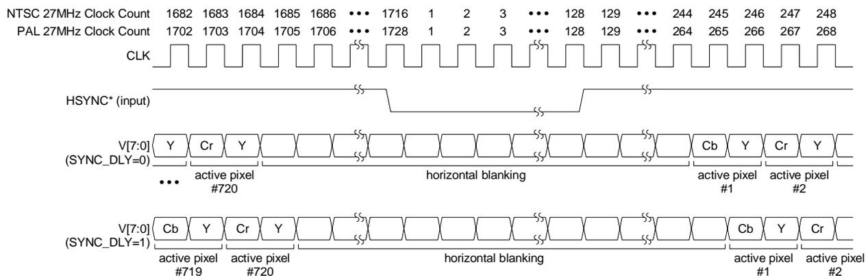
**Figure 6. CCIR601 Input Slave Mode Horizontal Timing**
