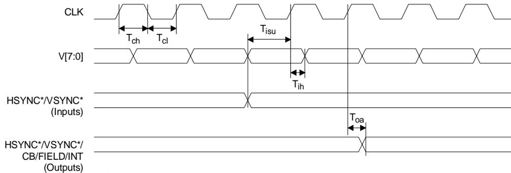
**Figure 1. Video Pixel Data and Control Port Timing**
