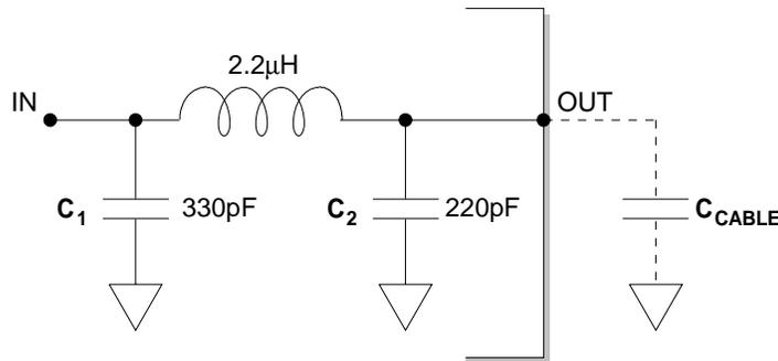
$C_2$  should be chosen so that  $C_1 = C_2 + C_{CABLE}$
