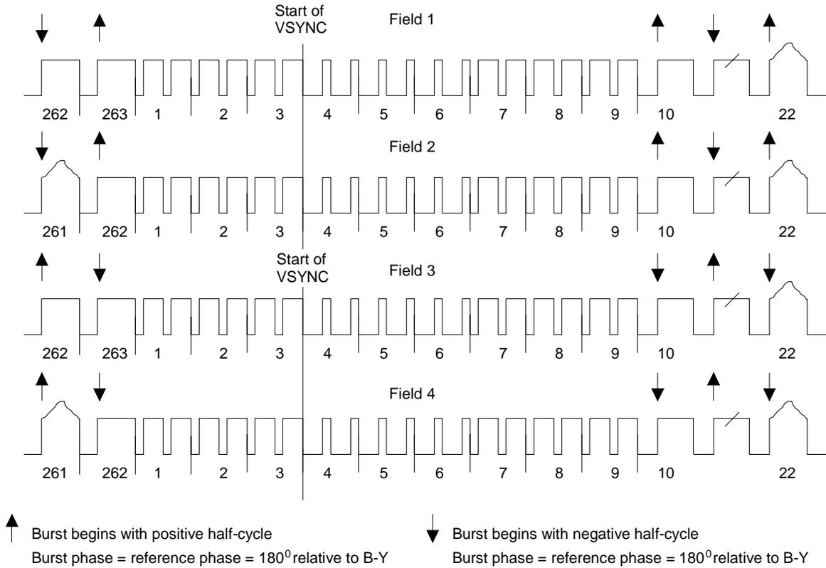
**Figure 12. NTSC Video Non-Interlaced Progressive Scan Timing**
