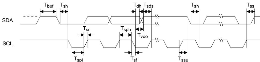
**Figure 2. I<sup>2</sup>C Host Port Timing**
