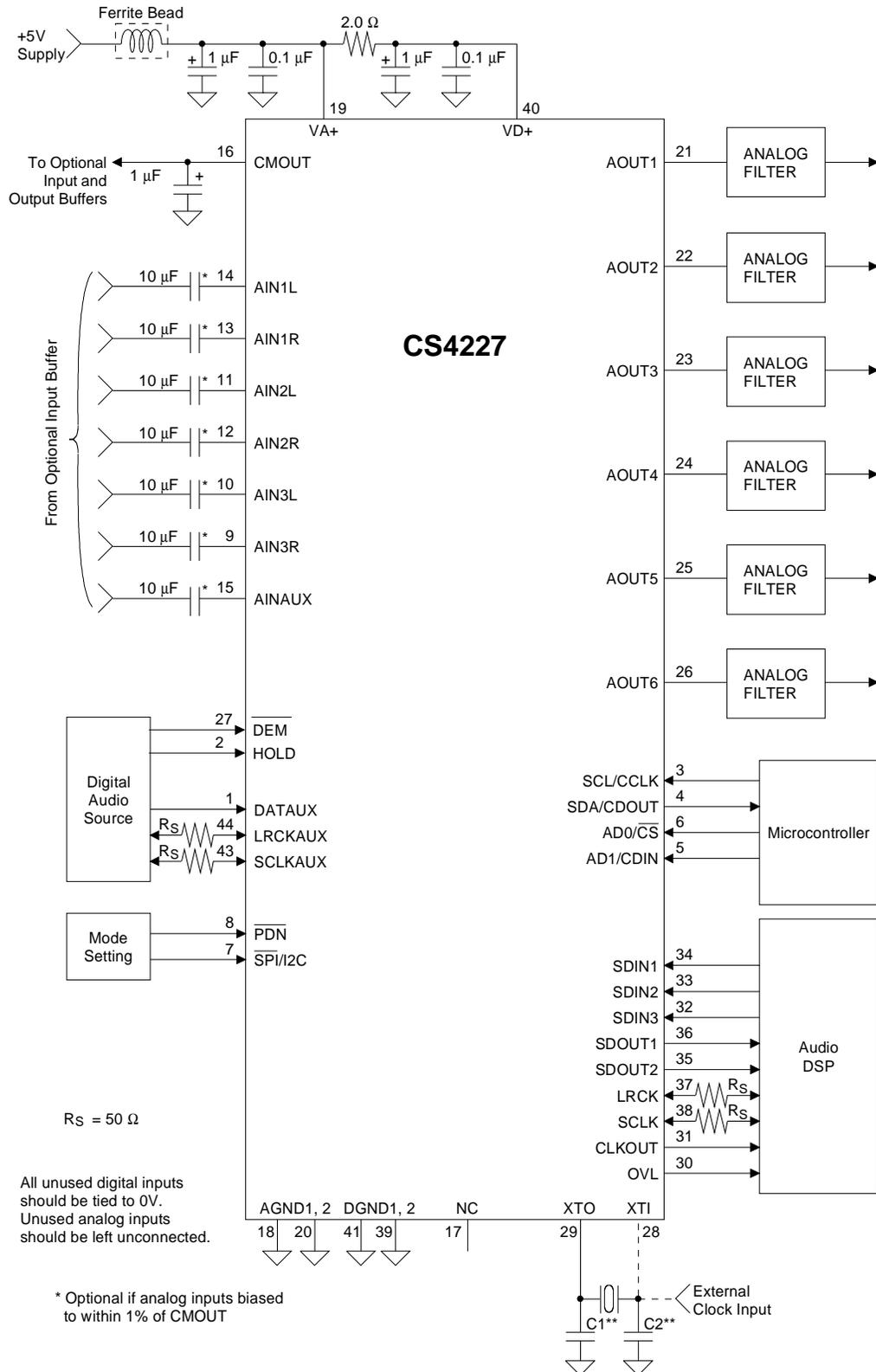
**Figure 5. Recommended Connection Diagram**
