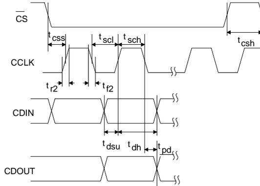
**Figure 3. Control Port SPI Mode**
