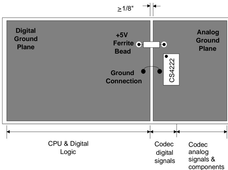
Note that the CS4222 is oriented with its digital pins towards the digital end of the board.
