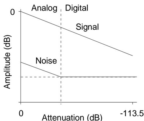
**Figure 5. Hybrid Analog/Digital Attenuation**
