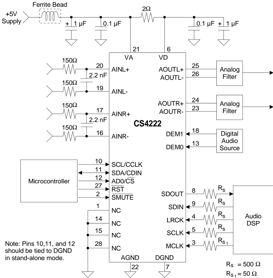
**Figure 1. Recommended Connection Diagram**
