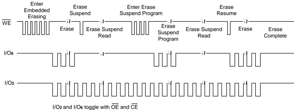
Note : Both I/O<sub>6</sub> and I/O<sub>2</sub> toggle with  $\overline{OE}$  or  $\overline{CE}$ . See the text on I/O<sub>6</sub> and I/O<sub>2</sub> in the section "Write Operation Statue" for more information.
