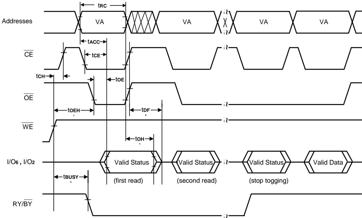
Note: VA = Valid Address; not required for  $I/O_6$ . Illustration shows first two status cycle after command sequence, last status read cycle, and array data read cycle.
