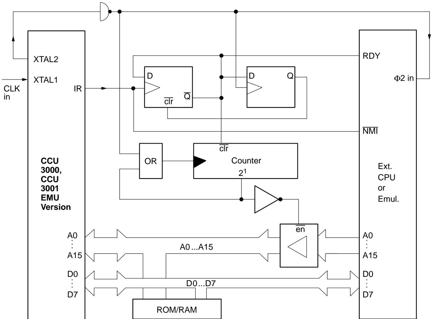
Fig. 2-12: Using an external CPU
