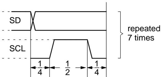
Fig. 2-21: Single bit on I<sup>2</sup>C bus
