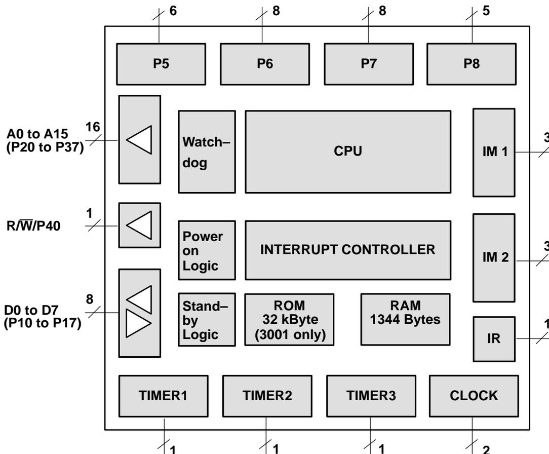
Fig. 1-1: CCU 3000, CCU 3001 block diagram
