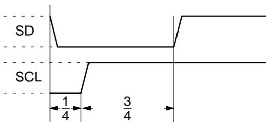
Fig. 2-22: Stop condition I<sup>2</sup>C bus
