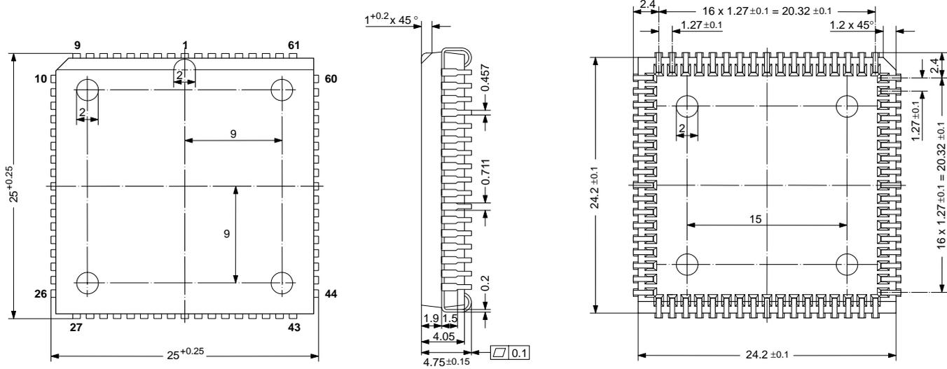
**Fig. 4-1: 68-Pin Plastic Leaded Chip Carrier Package (PLCC68)**
