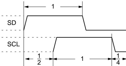
Fig. 2-20: Start condition I<sup>2</sup>C bus
