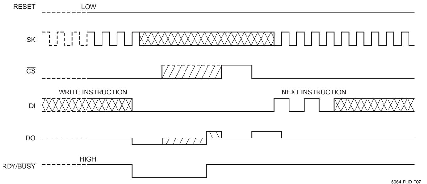
WRITE cycle. The RDY/ $\overline{\text{BSY}}$  pin will output the  $\overline{\text{BUSY}}$  status (LOW) one  $t_{\text{SV}}$  after the rising edge of the 32nd clock (the last data bit) and will stay LOW until the write cycle is complete. Then it will output a logical "1" until the next WRITE cycle. The RDY/ $\overline{\text{BSY}}$  output is not affected by the input of  $\overline{\text{CS}}$ .
