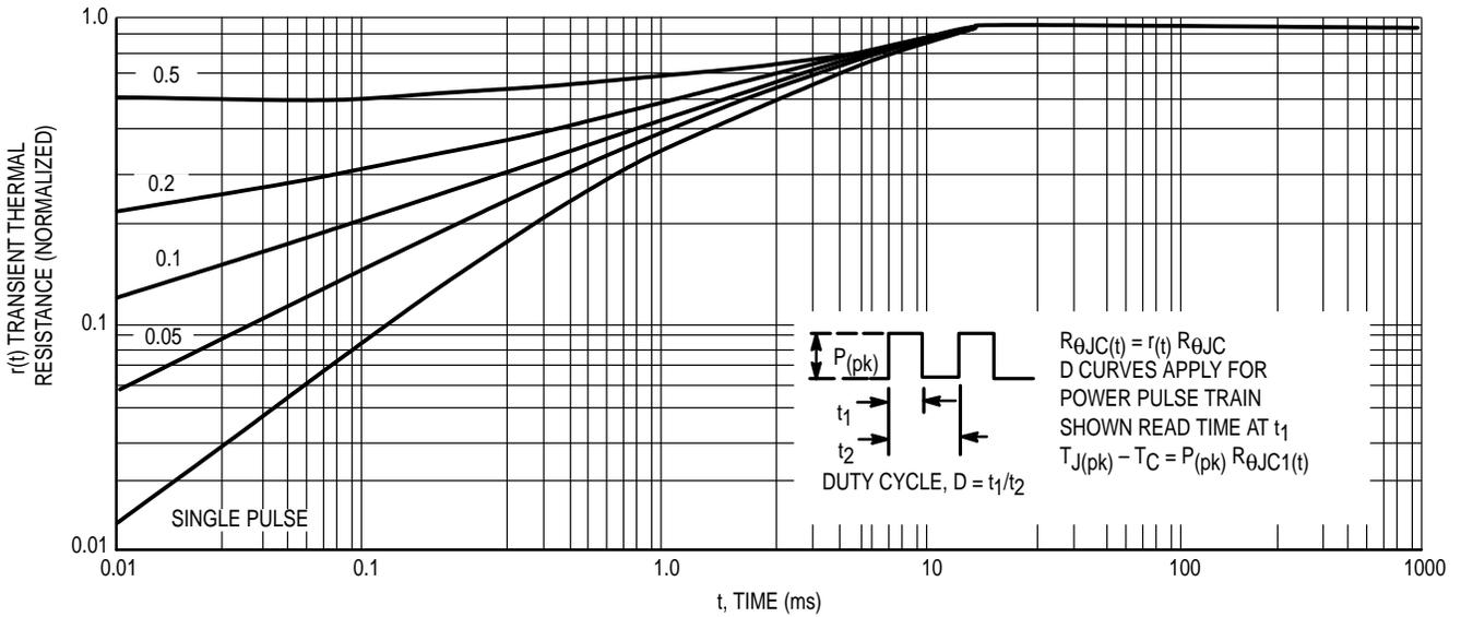
Figure 21. Typical Thermal Response ( $Z_{\theta JC}(t)$ ) for BUL44F
