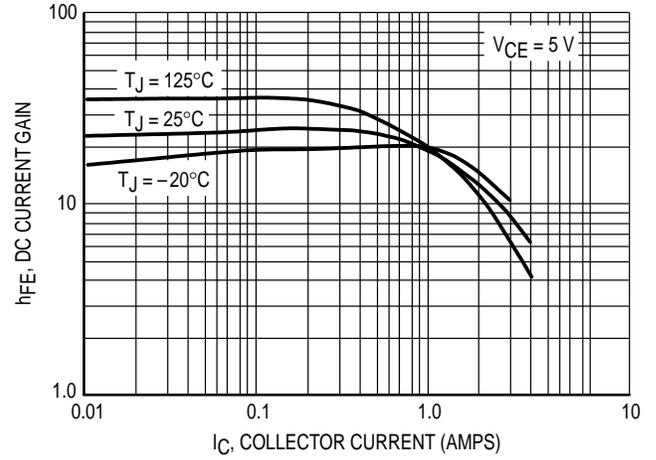
Figure 2. DC Current Gain at 5 Volts
