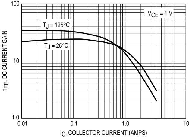
Figure 1. DC Current Gain at 1 Volt
