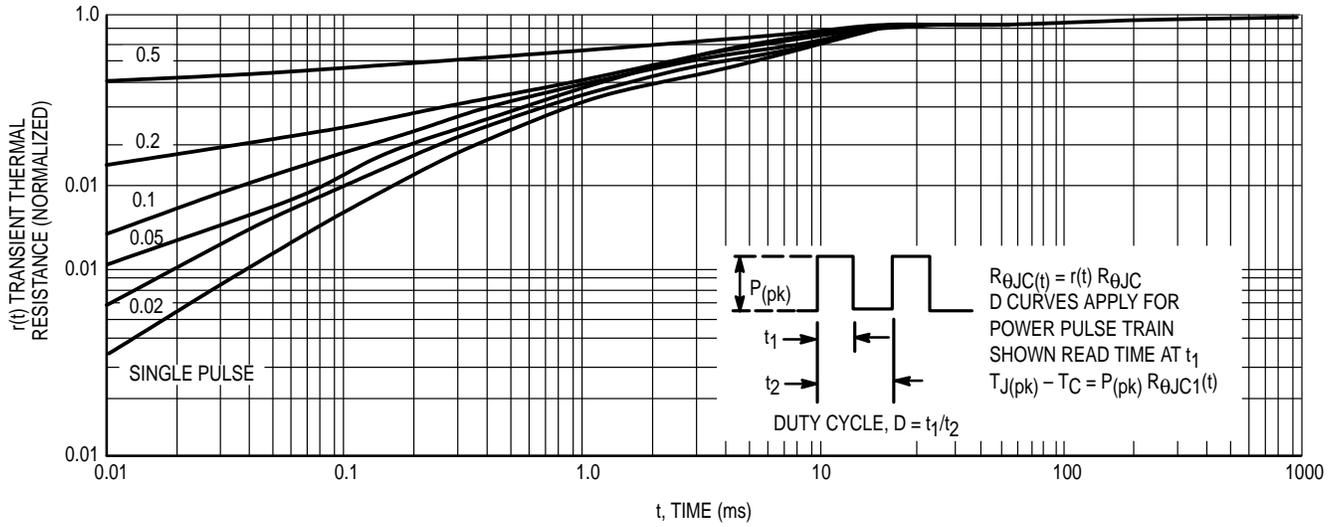
Figure 20. Typical Thermal Response ( $Z_{\theta JC}(t)$ ) for BUL44
