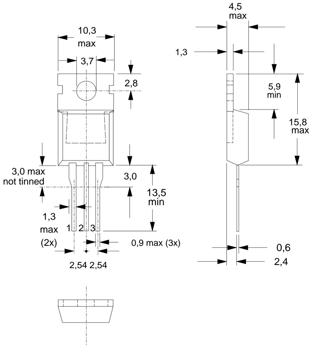
Fig.1. TO220AB; pin 2 connected to mounting base.
